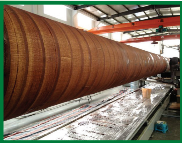
Bamboo fiber piping fabrication at Zhejiang Xinzhou Bamboo-based Composites Technology Co. Ltd.
